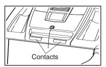
handrail—**avoid moving your hands**. When your pulse is detected, one or two dashes will appear in the right side of the display and then your heart rate will be shown. For the most accurate heart rate reading, continue to hold the contacts for about 15 seconds.
